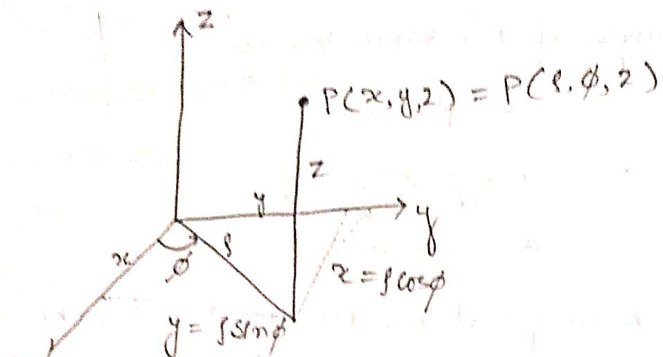
The relationship between the variables  $(x, y, z)$  of the Cartesian coordinate system and those of the cylindrical system  $(r, \phi, z)$
