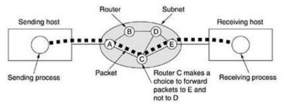
A stream of packets from sender to receiver.
